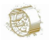
Hand Shield. An open face shield for manual excavation
