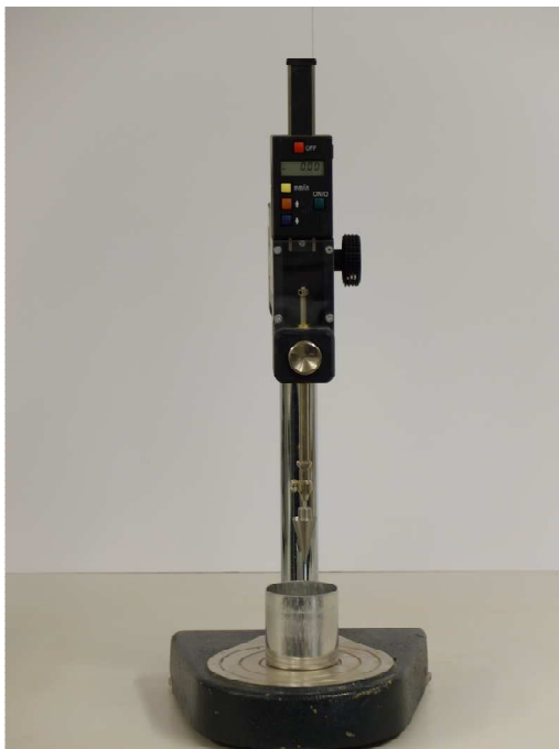
Figure 4.15 Fall cone apparatus for determination of liquid limit
