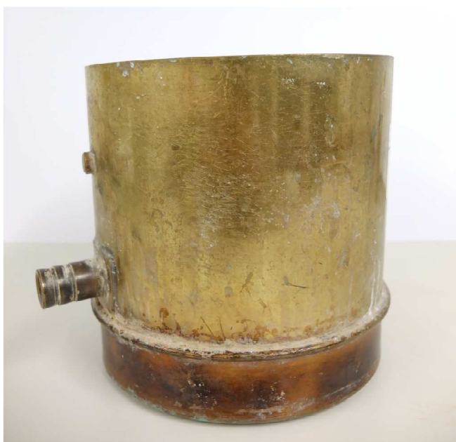
Figure 4.7 Adapted base pan for series 1 mixing test
