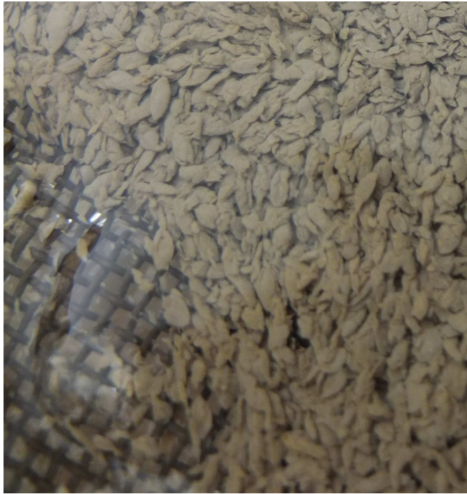
Figure 6.17 London clay, Maida Vale, 0.15% HydroCut mixing test.) Flocculated material on the 1.18 mm sieve
