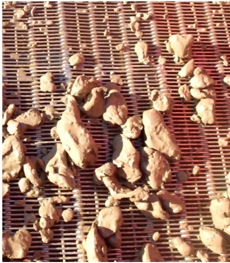
London clay cuttings on clay ball belt separator, mesh openings 3x50 mm
