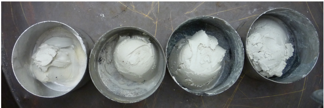
Figure 5.3 Samples after 30min vibration showing very little free water and a stiffer sample then would be seen from a decanting centrifuge (100, 50, 25, 10mg/l)
