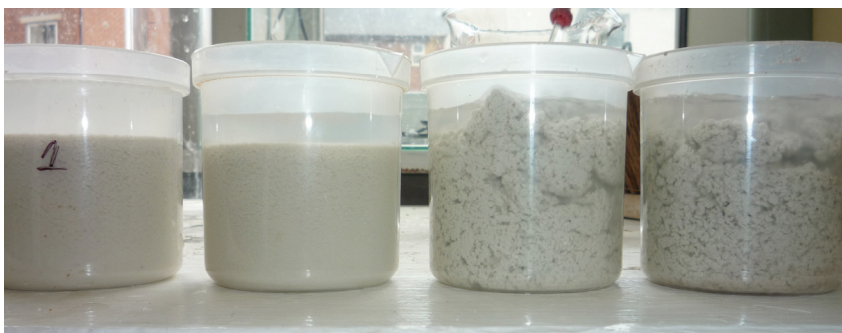
Figure 5.2 Variation in visible floc size 1-4 (10, 25, 50, 100\text{mg/l} )
