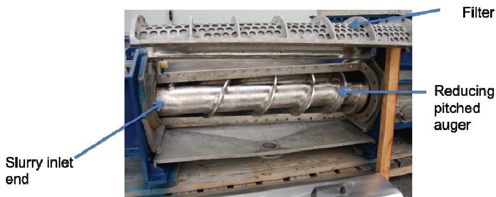
Figure 2.13 Internal workings of a screw press (Vincent Corp, 2008)
