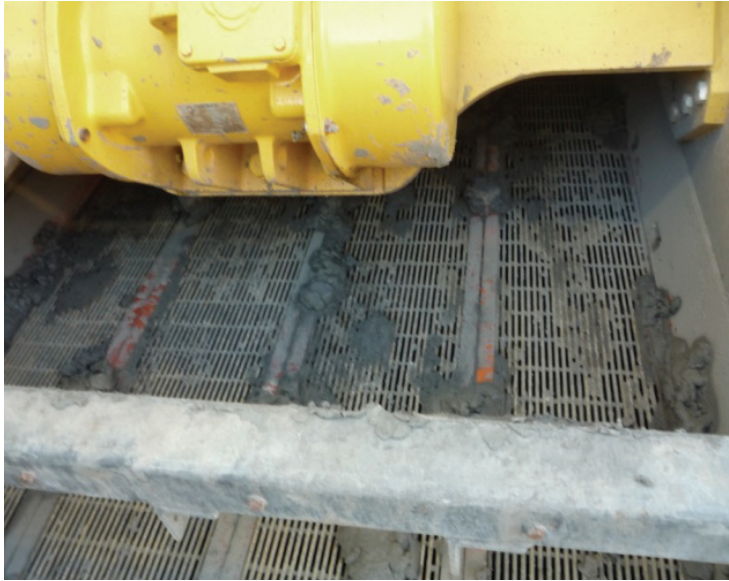
Figure 1.4 Primary shaker screen
