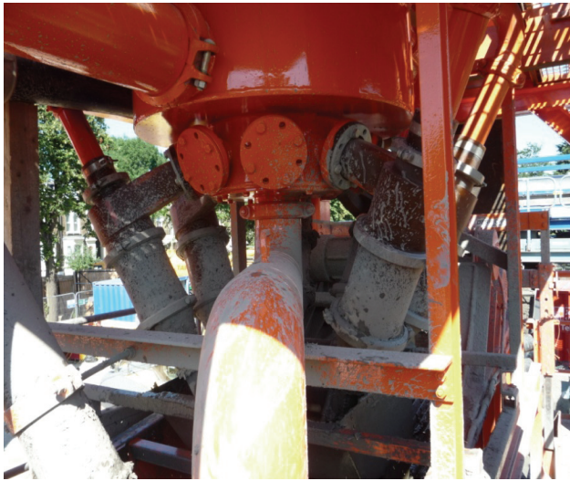
Figure 1.6 Bank of hydro-cyclones (150mm Ø)
