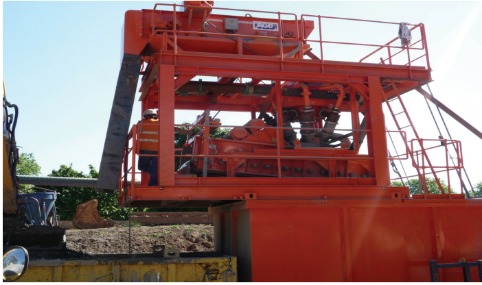
Figure 1.8 Shaker screen looking at the side and the bed
