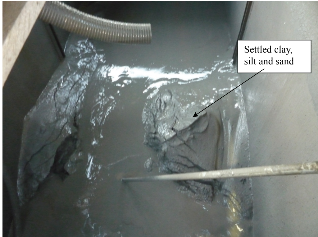
Figure 3.5 The bottom of the slurry tank using air agitation once the slurry had been removed for disposal
