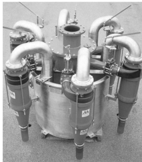
Figure 2- 8 A typical cross section of hydrocyclone and a set of six cyclones connected to a common feeding system (Tarleton and Wakeman, 2007)
