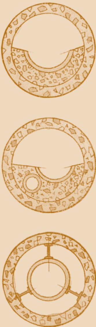
Typical reinverting & secondary lining detail
